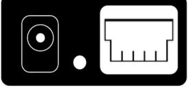
+5VDC Power Jack INT Line I<sup>2</sup>C Interface Connector
