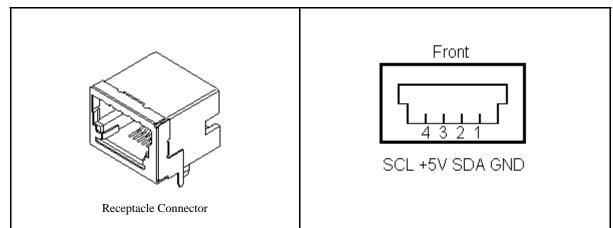
An I<sup>2</sup>C Interface Cable (White=SCL, Red=+5VDC, Green=SDA, Black=Ground) is provided to connect to a external I<sup>2</sup>C Bus. Since there is no standard I<sup>2</sup>C Bus connector, you may want to cut off one end of the cable and add a connector compatible with your target system.
