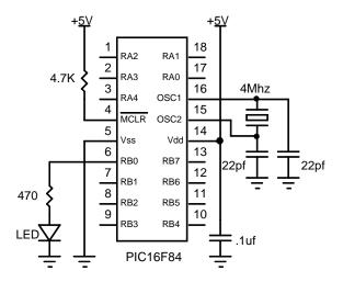
Build and double check this simple circuit on a breadboard and plug in the PICmicro MCU you just programmed. Our line of **PICProto** prototyping boards is perfect for this kind of thing.
