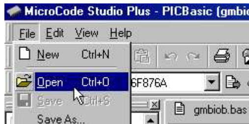
FIGURE 38: LOADING SOURCE FILE WITH MICROCODE STUDIO + PIC BASIC
