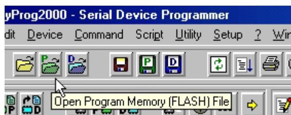
FIGURE 33: LOADING FILE TO PROGRAM WITH PONYPROG
