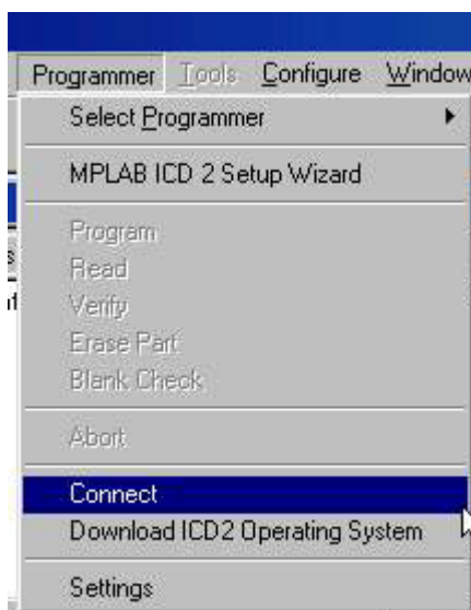
FIGURE 22: CONNECTION TO MP LAB® ICD 2
