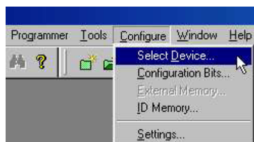
FIGURE 21: DEVICE SELECTION WITH MP LAB® ICD 2
