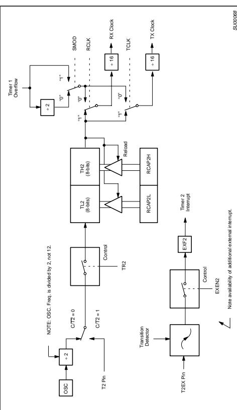
Figure 4. Timer 2 in Baud Rate Generator Mode
