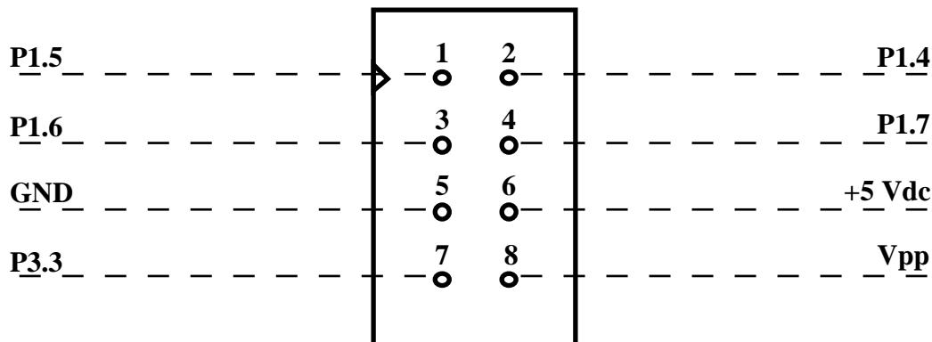
FIGURE 17: CN5 - CPU I/O LINES AND PROGRAMMING VOLTAGE CONNECTOR
