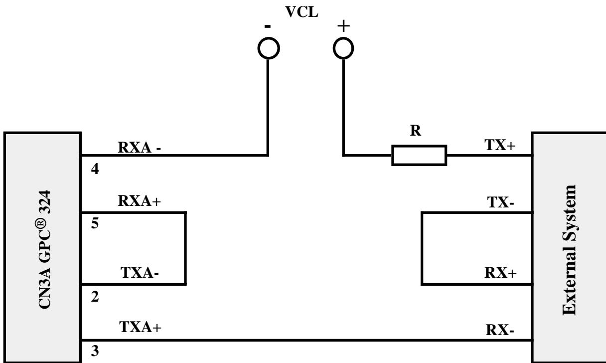
**FIGURE 15: 2 WIRES CURRENT LOOP POINT TO POINT CONNECTION EXAMPL**
