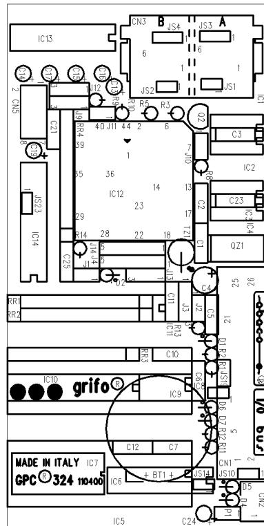
FIGURE 20: COMPONENTS MAPS (SOLDERING SIDE )
