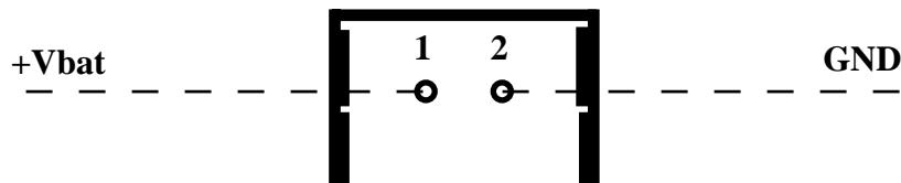
FIGURE 4: CN2 - EXTERNAL BACK UP BATTERY CONNECTOR
