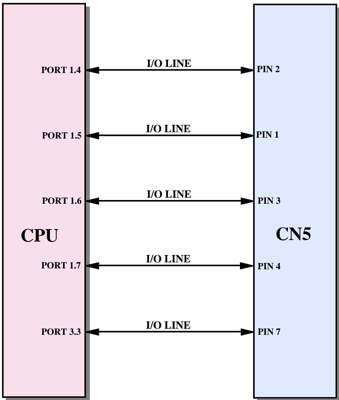
FIGURE 18: I/O LINES CONNECTION DIAGRAM
