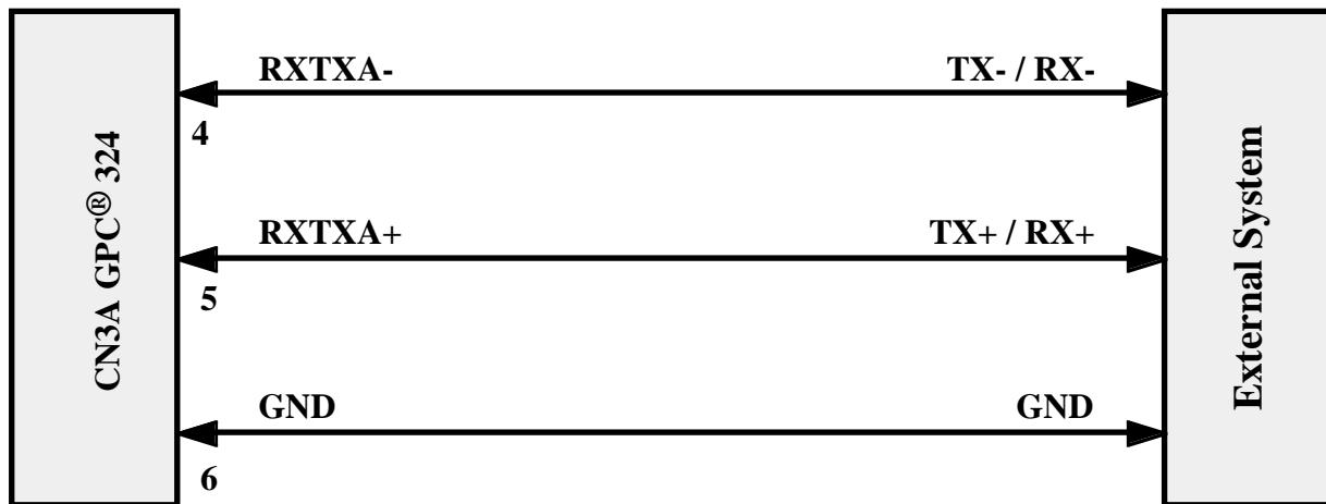
**FIGURE 12: RS 485 POINT TO POINT CONNECTION EXAMPLE**
