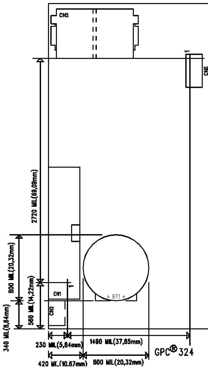
FIGURE A1: MODULE DIMENSION FOR PIGGY BACK MOUNTING
