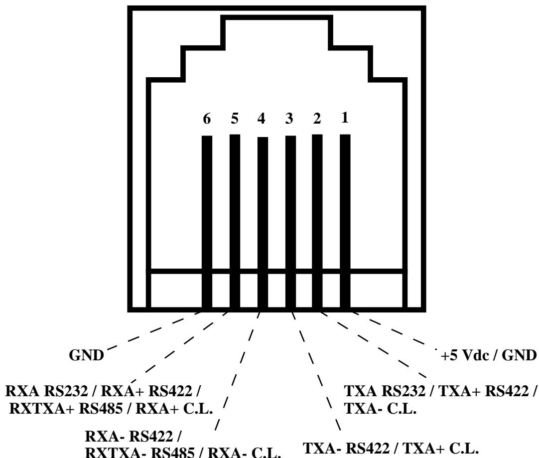
**FIGURE 6: CN3A - SERIAL LINE A CONNECTOR**
