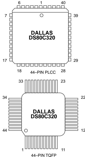
The DS80C320 is pin compatible with all three packages of the standard 80C32 and offers the same timer/counters, serial port, and I/O ports. In short, the DS80C320 is extremely familiar to 8051 users but provides the speed of a 16-bit processor.
