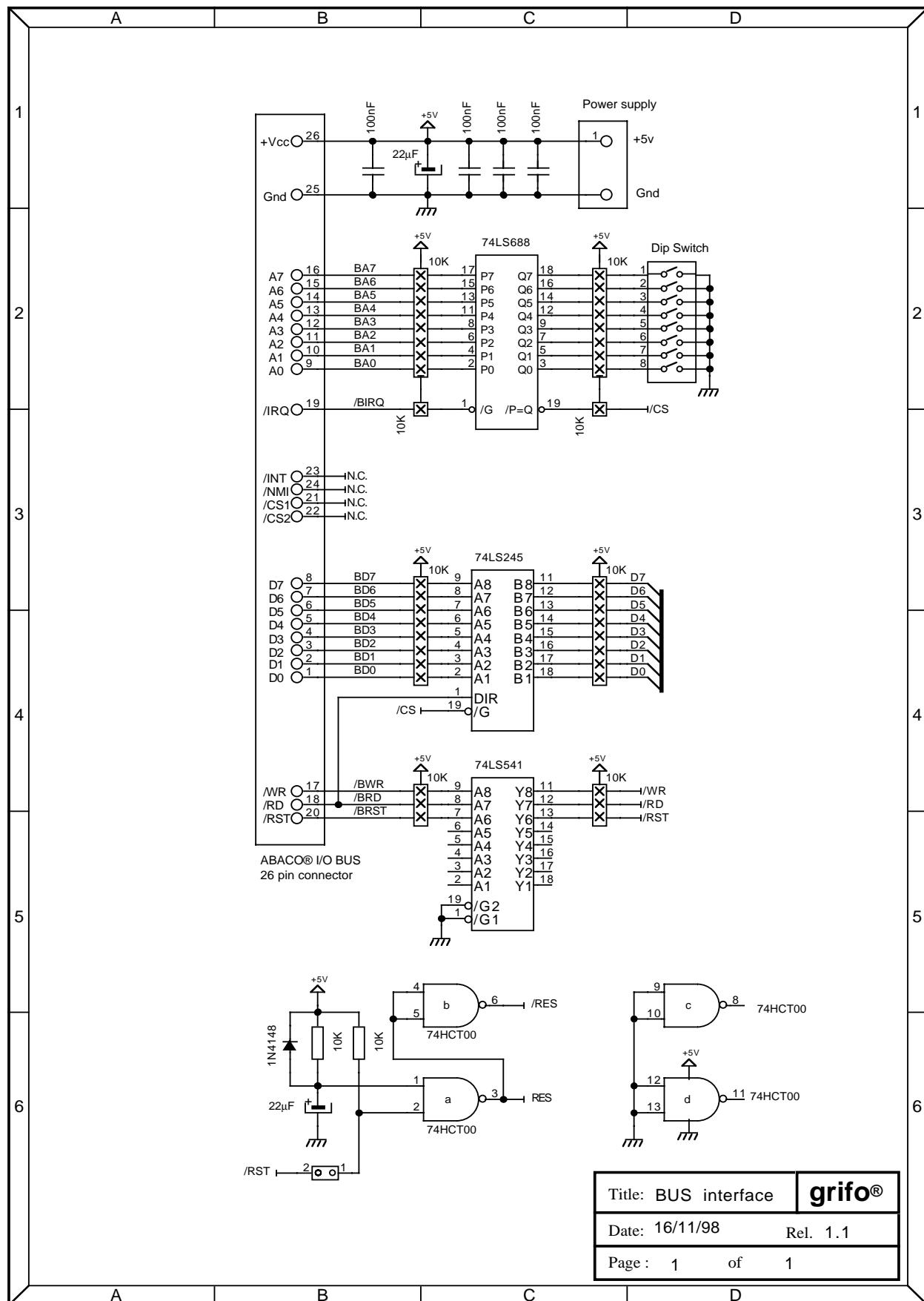
FIGURE C7: BUS INTERFACE ELECTRIC DIAGRAM
