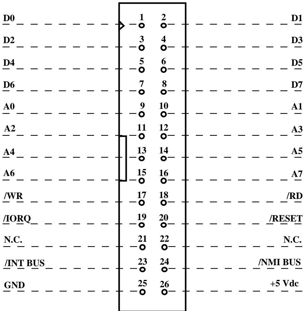
FIGURE 5: CN1 - ABACO® I/O BUS CONNECTOR
