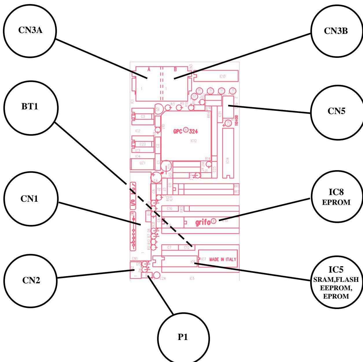
FIGURE 7: P1, MEMORIES, BATTERY, CONNECTORS LOCATION
