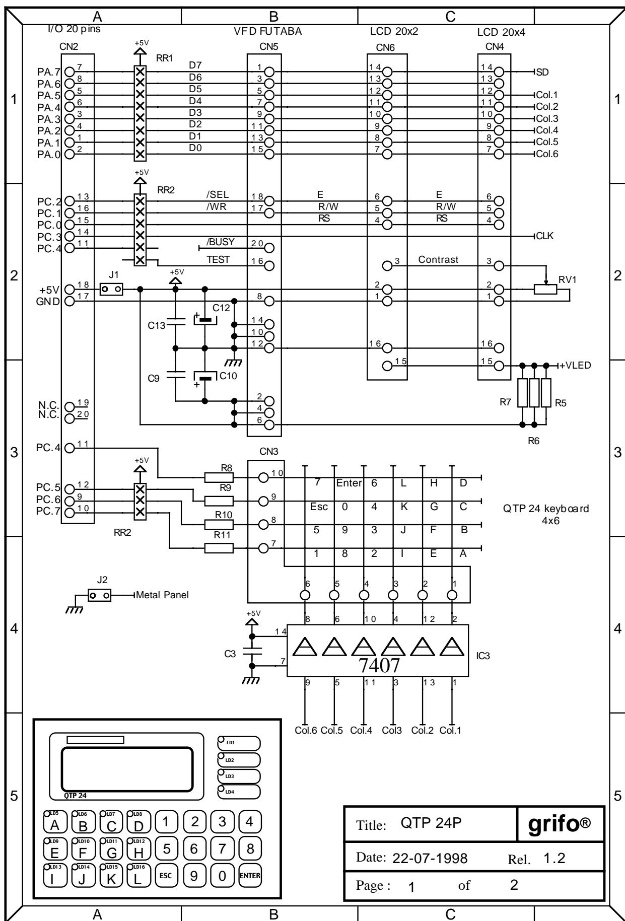
FIGURE C4: QTP 24P ELECTRIC DIAGRAM (1 OF 2)
