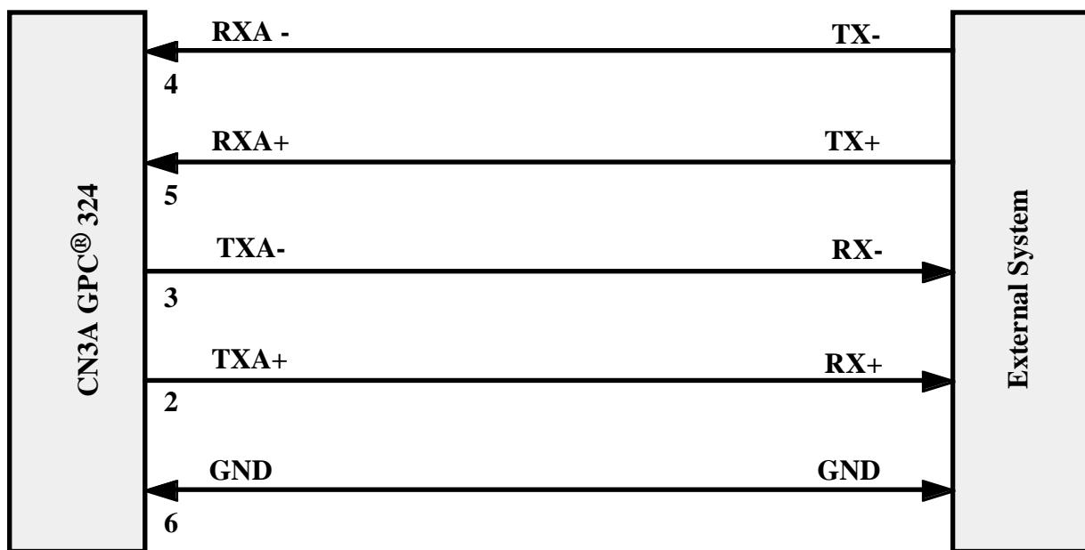
**FIGURE 11: RS 422 POINT TO POINT CONNECTION EXAMPLE**
