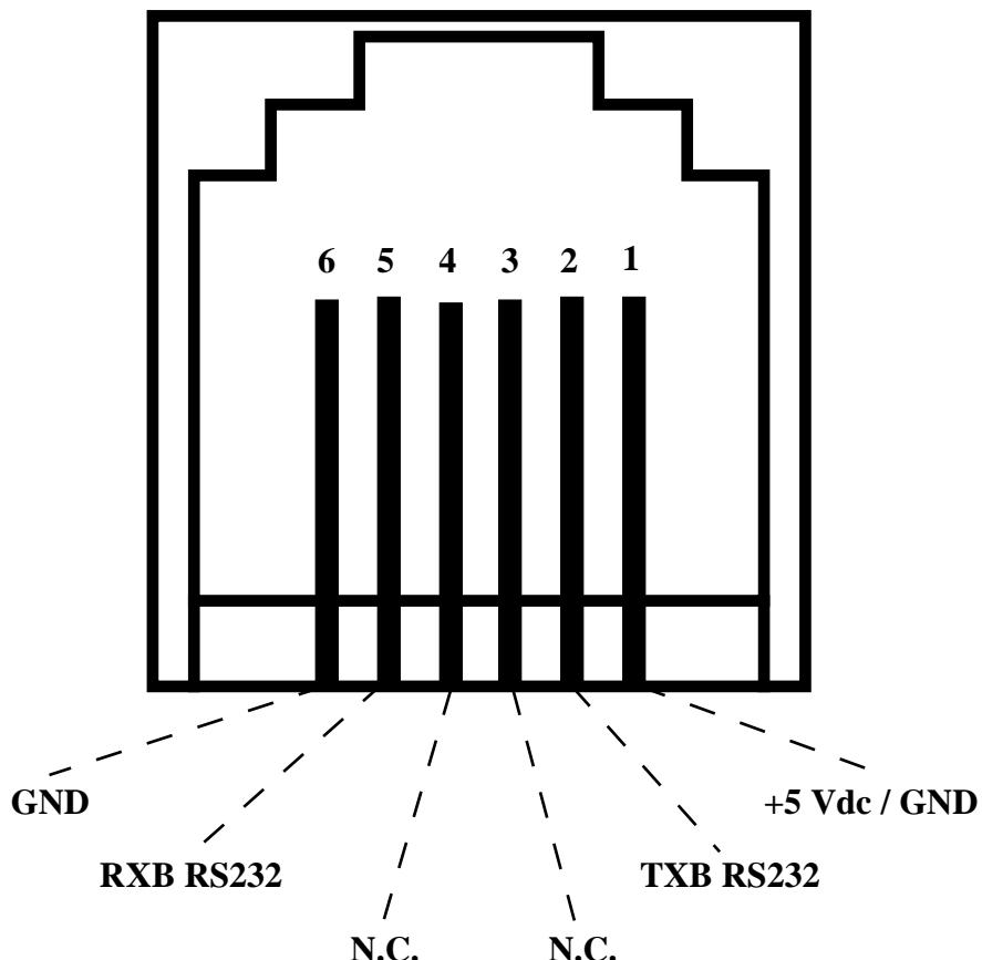
FIGURE 8: CN3B - SERIAL LINE B CONNECTOR
