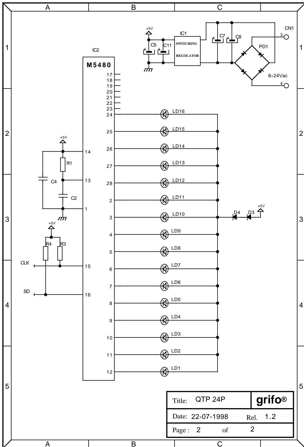
FIGURE C5: QTP 24P ELECTRIC DIAGRAM (2 OF 2)
