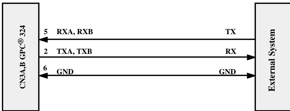
**FIGURE 10: RS 232 POINT TO POINT CONNECTION EXAMPLE**
