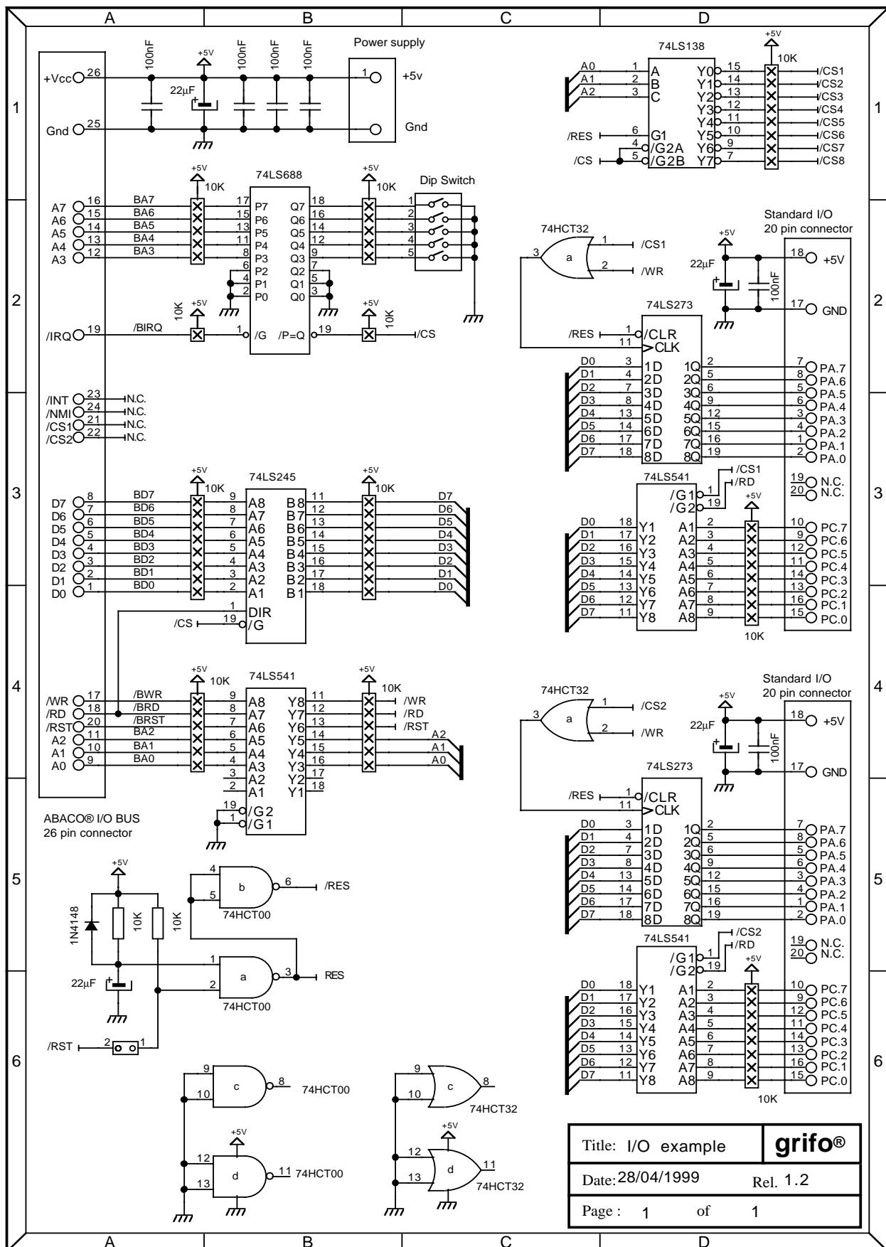
FIGURE C6: ABACO® I/O BUS INPUT OUTPUT ELECTRIC DIAGRAM
