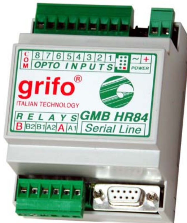
FIGURE 6: PHOTO OF GMB HR84 WITH CONTAINER
