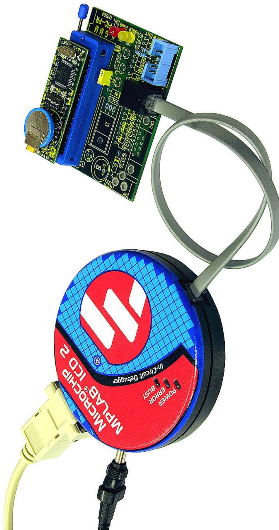
FIGURE 19: IMAGE OF GMM 4620 ON A GMM PIC-PR CONNECTED TO MP LAB® ICD 2
