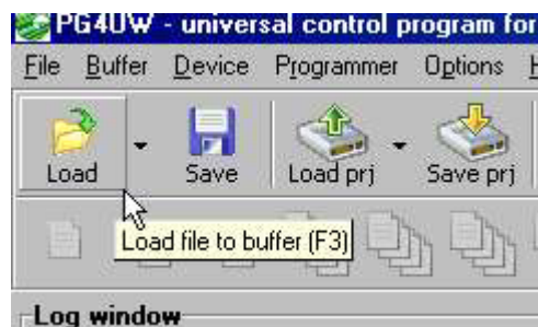
FIGURE 21: LOADING FILE TO PROGRAM WITH MP PIK+
