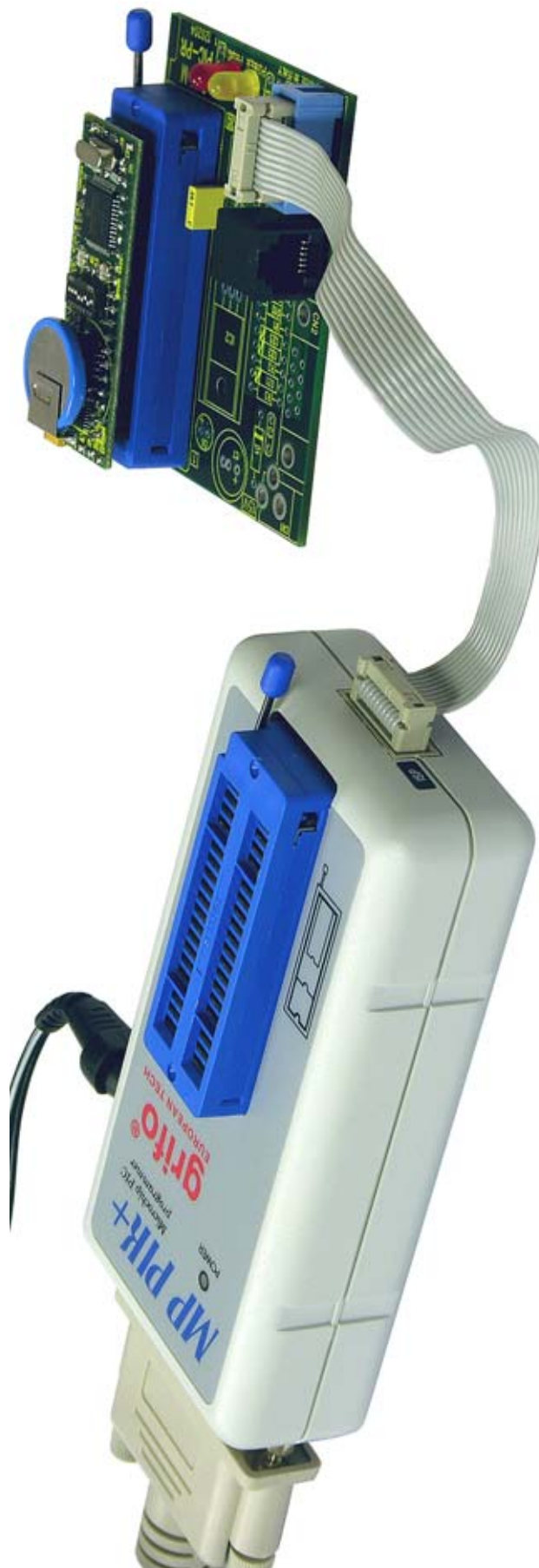
FIGURE 22: IMAGE OF GMM 4620 ON A GMM PIC-PR CONNECTED TO MP PIK+
