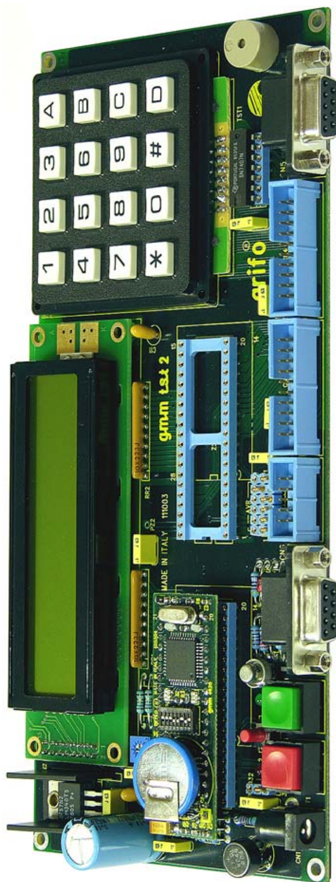
FIGURE 11: DEVELOPMENT BOARD GMM TST 2 WITH A GMM 4620 INSTALLED
