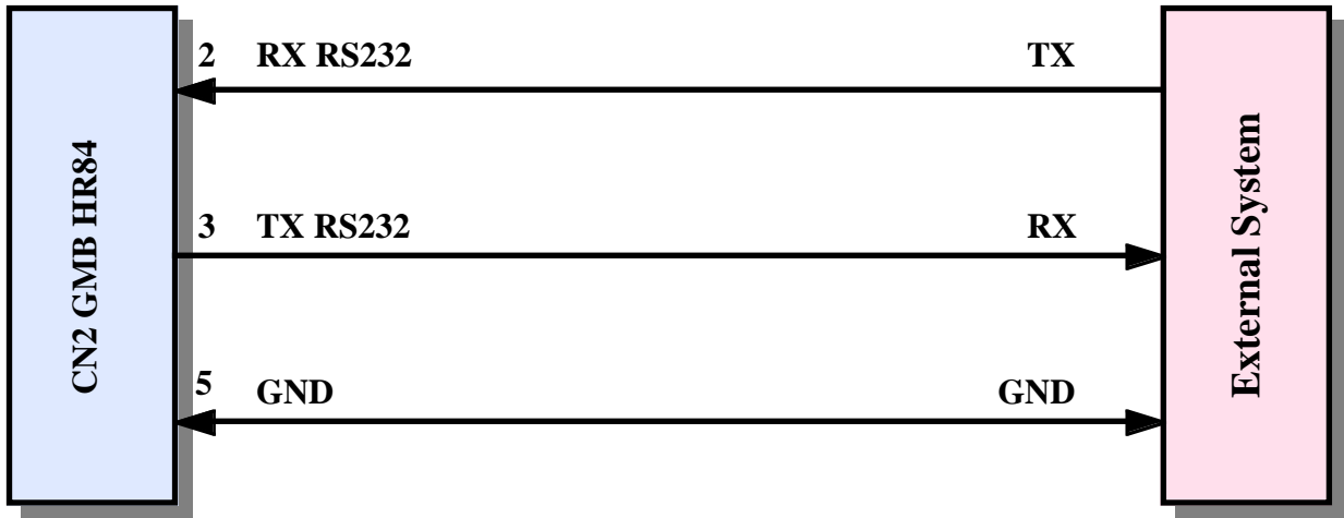
FIGURE 12: RS 232 POINT TO POINT CONNECTION EXAMPLE
