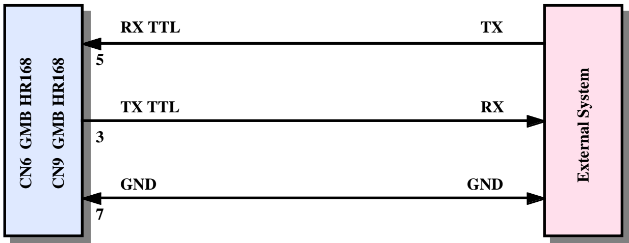
FIGURE 12: TTL POINT TO POINT CONNECTION EXAMPLE
