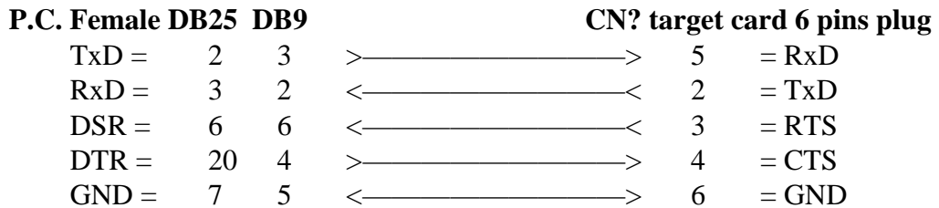
FIGURE 4: SERIAL CABLE BETWEEN P.C. AND TARGET CARD 6 PINS PLUG CONNECTOR
