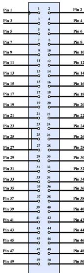
FIGURE 32: CN1 OF FBC 35 CONNECTION DIAGRAM
