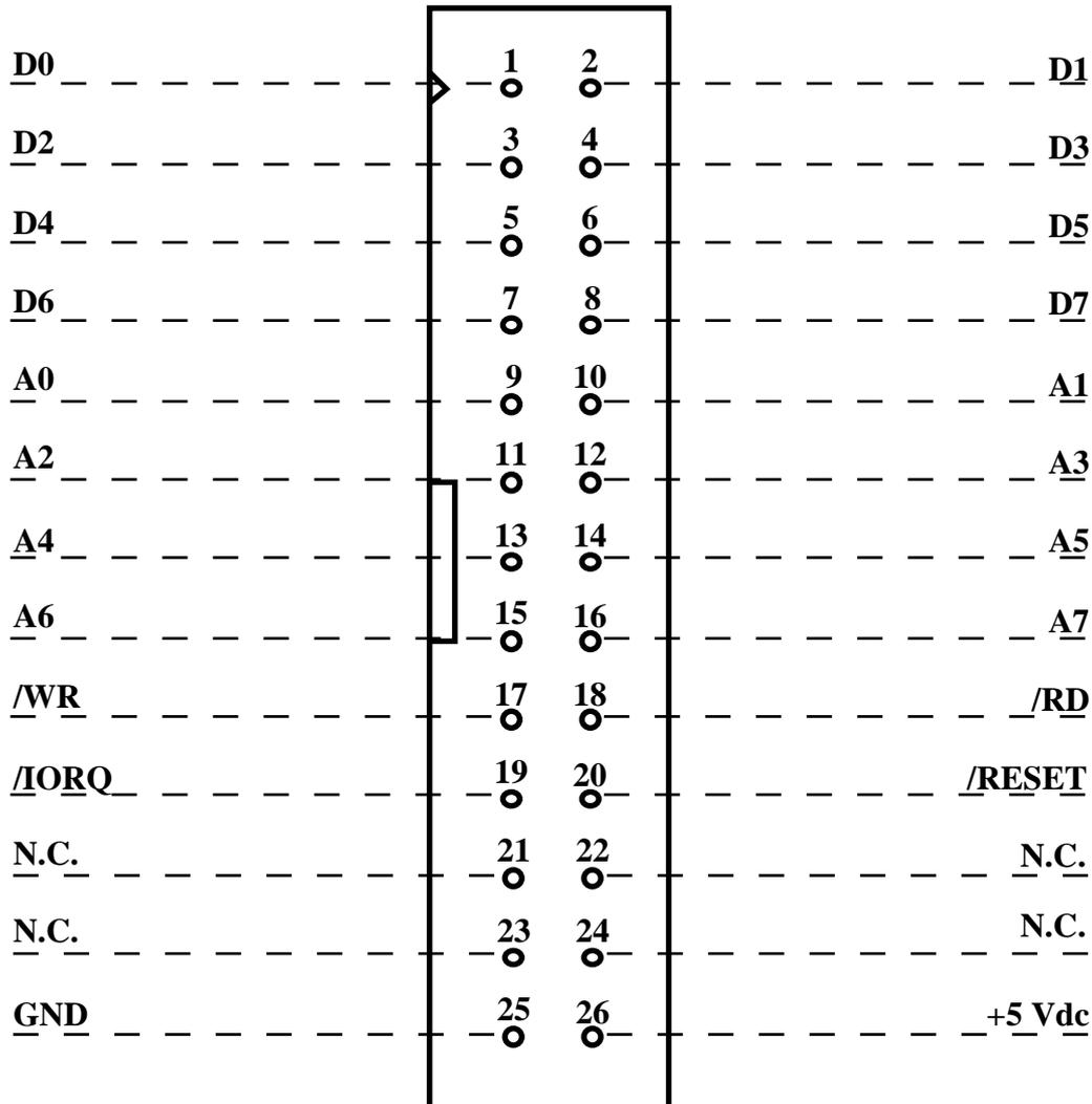
FIGURE 4: CN1 - ABACO® I/O BUS CONNECTOR
