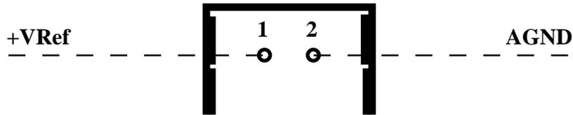
**FIGURE 6: CN2 - EXTERNAL REFERENCE VOLTAGE CONNECTOR**
