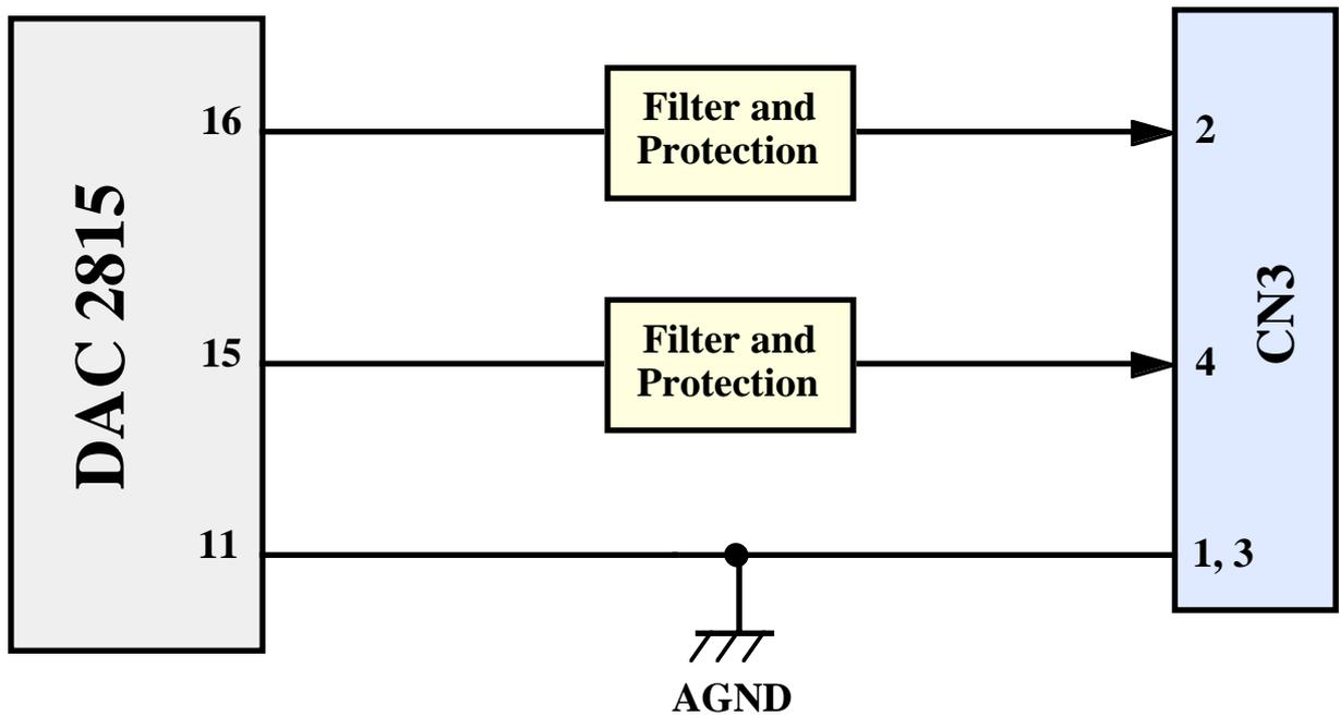
**FIGURE 3: ANALOG OUTPUTS BLOCK DIAGRAM**
