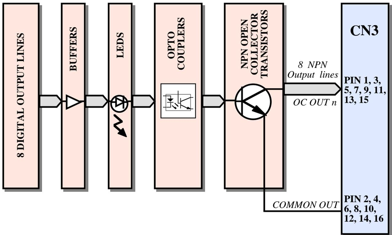
**FIGURE 10: DIGITAL OUTPUTS BLOCK DIAGRAM**
