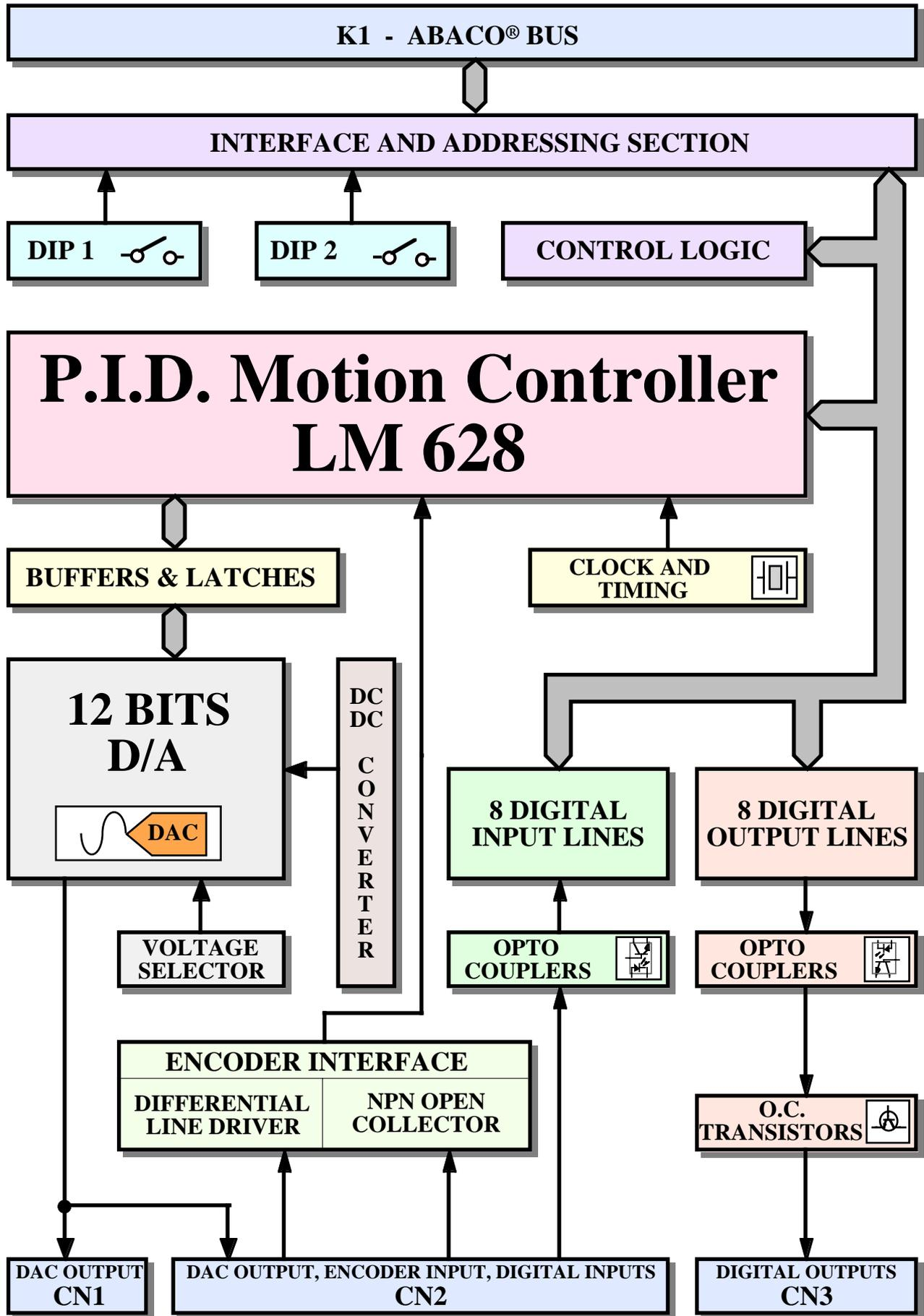
FIGURE 1: BLOCK DIAGRAM
