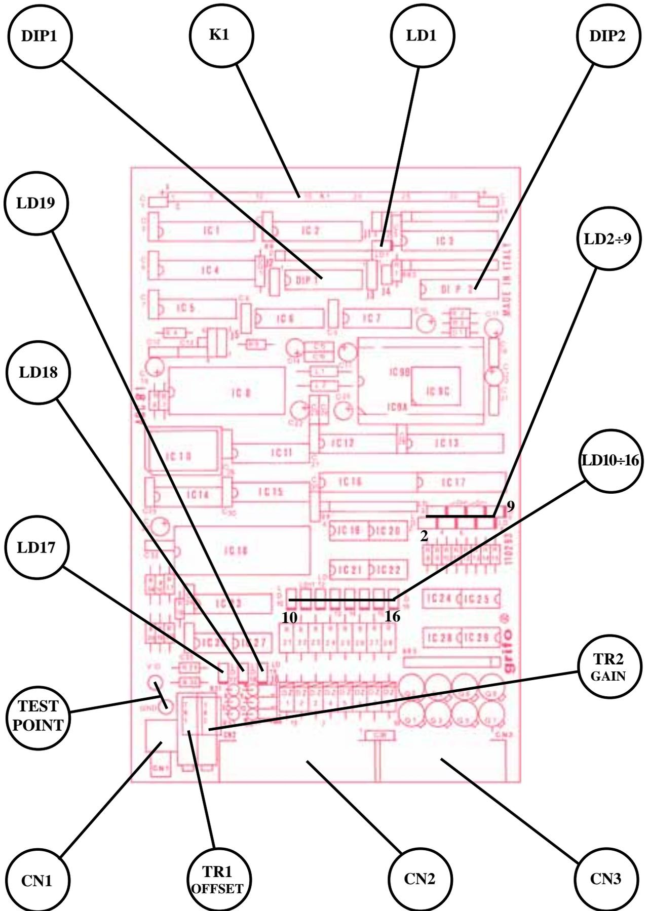
FIGURE 8: CONNECTORS, LEDs, DIP SWITCHES, ETC. LOCATION
