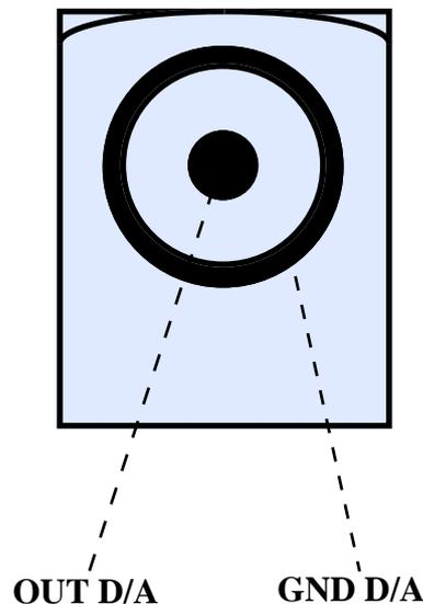
**FIGURE 3: CN1 - D/A ANALOG OUTPUT CONNECTOR**
