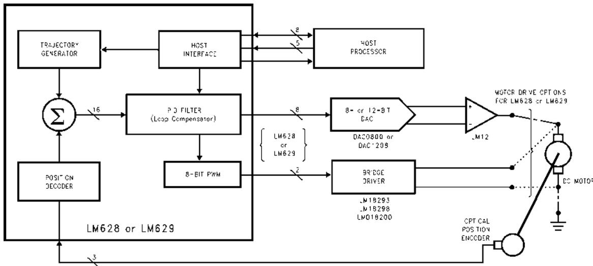
FIGURE 1. LM628 and LM629 Typical System Block Diagram
