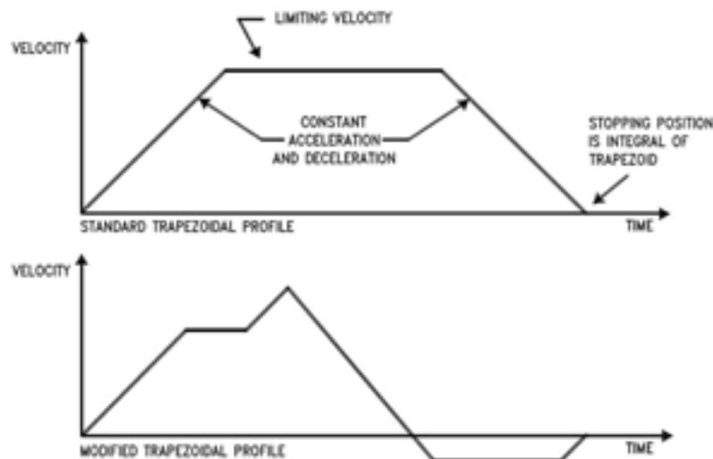
**FIGURE 22: VELOCITY PROFILES**
