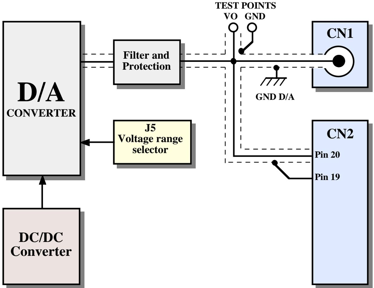
FIGURE 4: D/A SECTION BLOCK DIAGRAM
