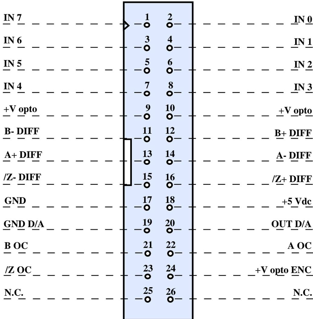
FIGURE 5: CN2 - ENCODER, ANALOG OUTPUT AND DIGITAL INPUTS CONNECTOR
