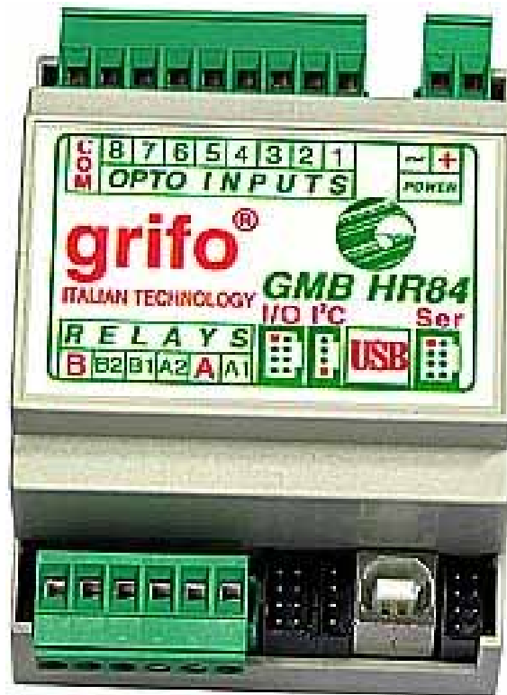
GMB HR84 with 8 Optocoupled Inputs and 4 Output Relays.
