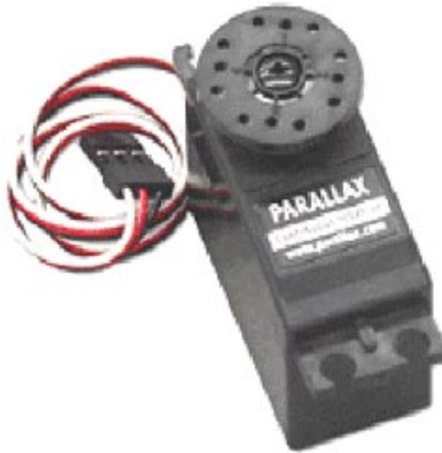
Continuous Rotation Servomotor Capable to Rotate over the 360°.
