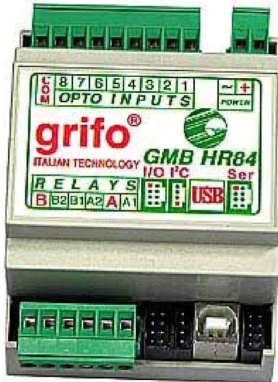
A GMB HR84 with 8 Optocoupled Inputs and 4 Relays Outputs.
